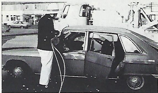
Spreading window space with the jaws
