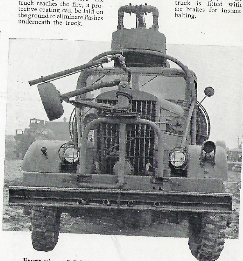
Front view of "Cardox" Class 150 Fire Truck, showing front nozzle and foam gun, with control mechanism. Also, linear ground sweep nozzle and four fixed foam guns below bumper. The boom is not extended in this illustration, but rests across top of truck (see also page 14).
